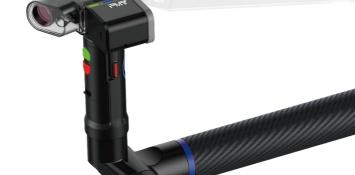
The PMT GAMMA 8-Axis is a complete rotary axis that can be directly connected to the GAMMA ARM. This integration enables a fully enclosed, high-accuracy add-on axis to the portable arm, saving time and effort during hardware setup. Unlike turntables, the 8-Axis is fully transparent to the measurement software and requires no software upgrades.
